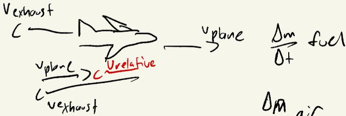
$$\begin{aligned} \text{Thrust} &= \text{fuel part} + \text{air part} \\ &= \frac{\Delta m}{\Delta t} \text{ fuel} (v_{\text{ejected}}) + \frac{\Delta m}{\Delta t} \text{ air} (v_{\text{relative}}) \end{aligned}$$
